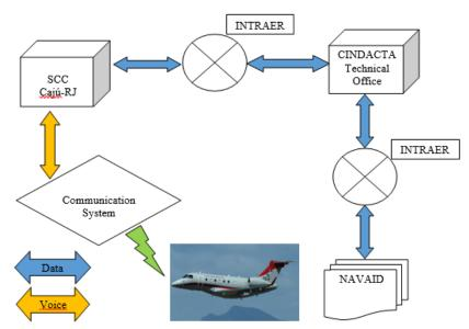
Figure 2-Galeão Basic Operation Diagram
