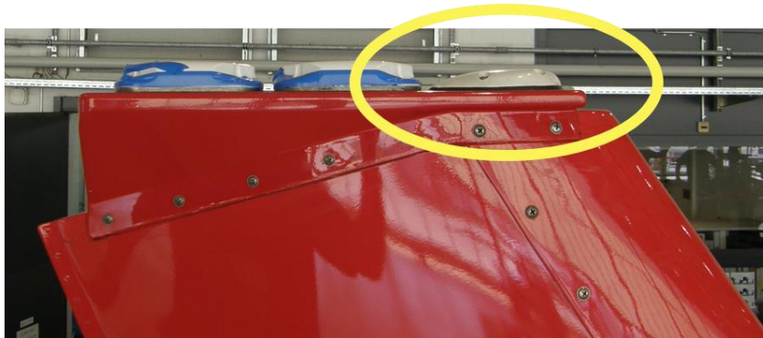
Figure 9: FIS GNSS Antenna, Side View
