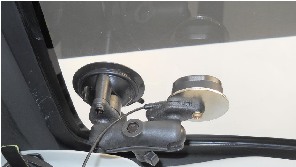
Figure 1: GNSS antenna in portable installation
