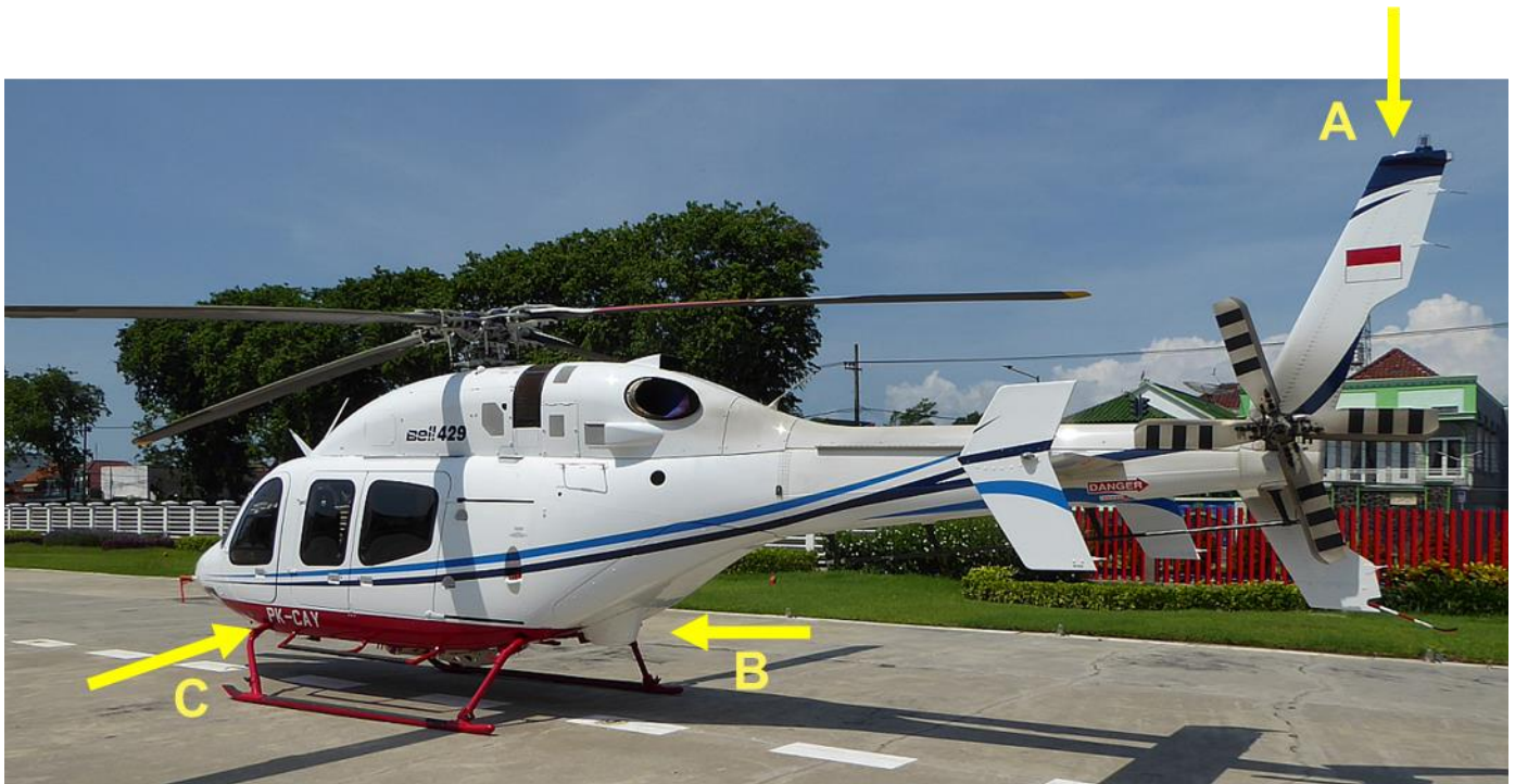
Figure 13: FIS Antenna Installations
