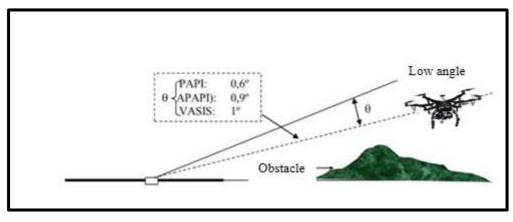
Fig. 8 - RPAS Obstacle Clearance in the Visual Navaid Flight Inspection Concept.
