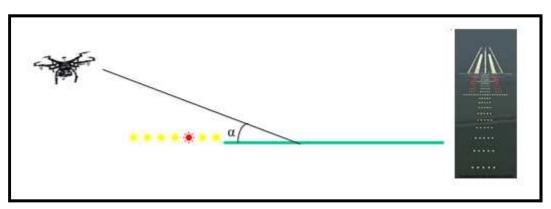
Fig. 9 - RPAS Operation, Intensity and Brightness of Lights of the ALS Flight Inspection Concept.
