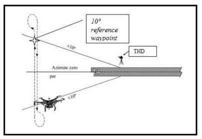
Fig. 7 – RPAS Angular Coverage in the Visual Navaid Flight Inspection Concept.
