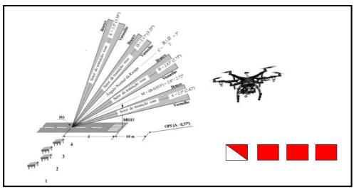
Fig. 6 - RPAS Transition Angle Inspection Concept.
