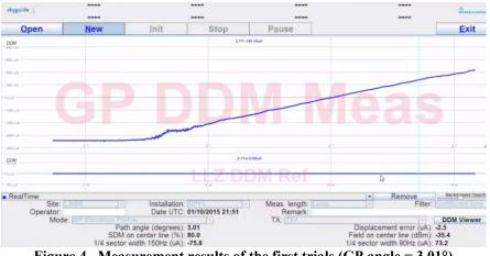
Figure 4. Measurement results of the first trials (GP angle = 3.01°)
