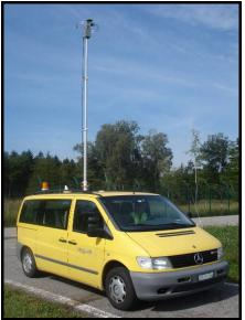
Figure 5. Measurement Vehicle in the Localizer Configuration
