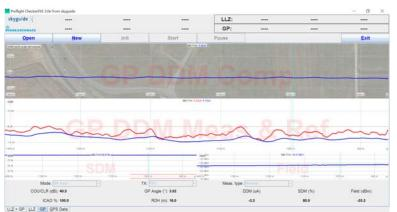
Figure 15. The Preflight Checker software in the Mini Approach mode: the Glide Path only window
