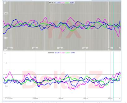
Figure 22. Assessment of the UAV flight accuracy and repeatability (zoom: +/- 2 m)
