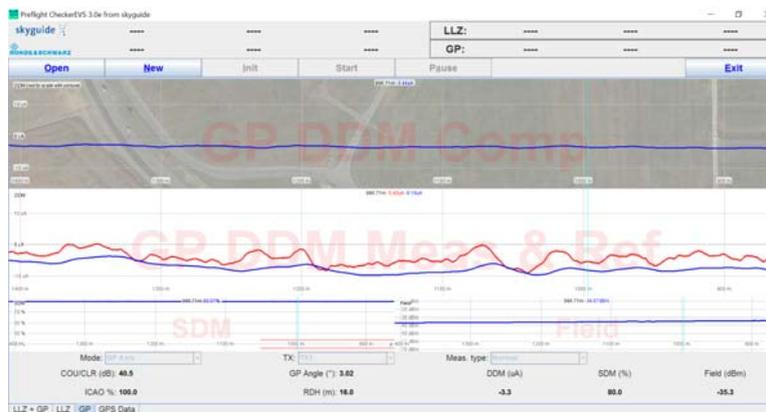
**Figure 15. The Preflight Checker software in the Mini Approach mode: the Glide Path only window**
