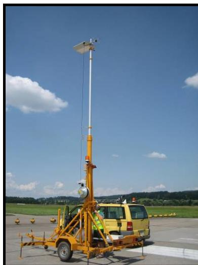
**Figure 6. Telescopic Mast at the runway threshold**
