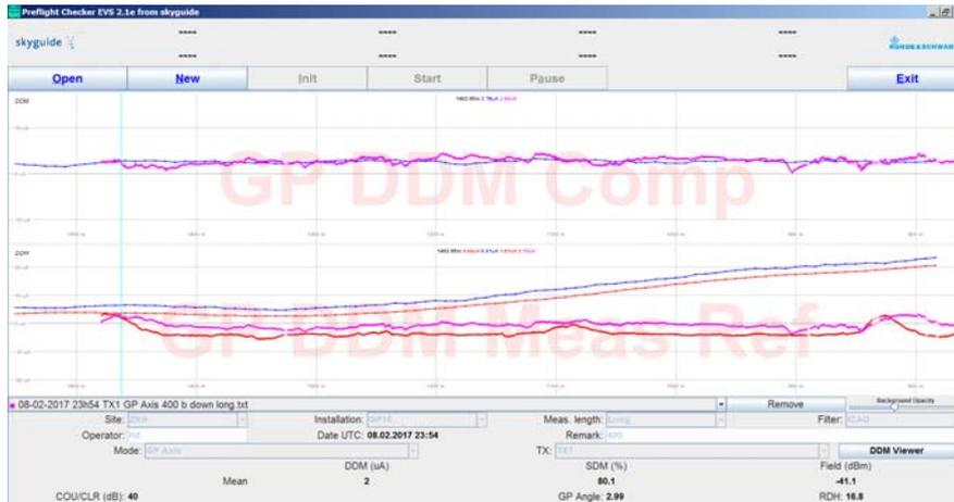
Figure 24. Correlation between flight check (in blue) and UAV measurements (in pink) for Mini Approach
