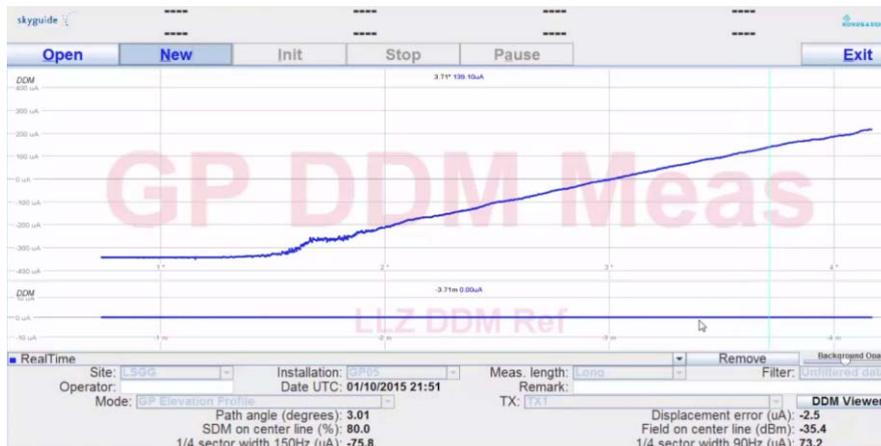
Figure 4. Measurement results of the first trials (GP angle = 3.01°)
