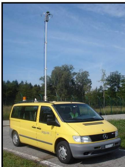
Figure 5. Measurement Vehicle in the Localizer Configuration
