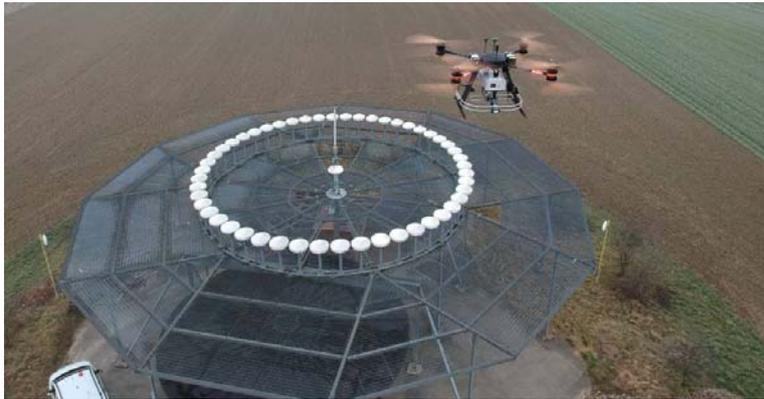
**Figure 25. The UAV multicopter over a VOR**
