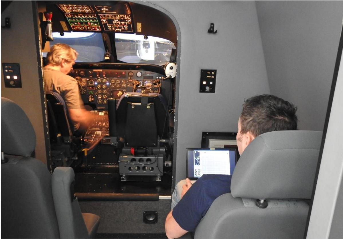
FIS simulation computer inside the motion cabin
