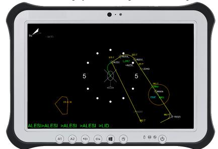
Picture shows a portable cockpit moving map display with procedure guidance
