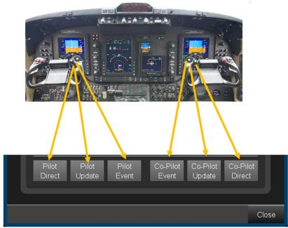
Picture shows a cockpit and the according FIS simulation control window
