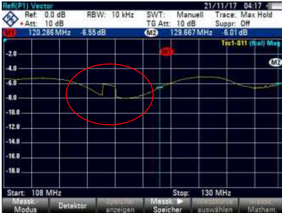
Figure 18: Glitch proving intermittent electrical disconnection
