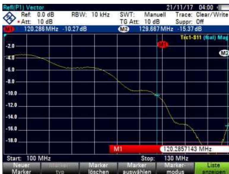
Figure 16: VSWR plot of top antenna
