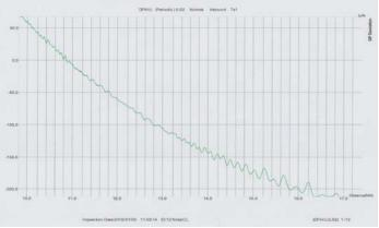
Figure 4 An unacceptable GP clearance curve
