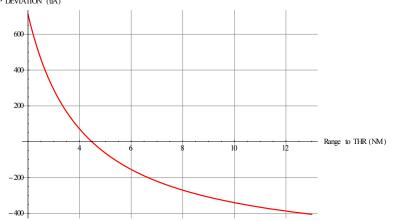
Figure 5 A GP clearance curve derived from theoretical calculation
