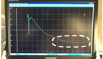
Figure 11 A GP Clearance Curve whose DDM is only  $-240\mu A$  at low angle
