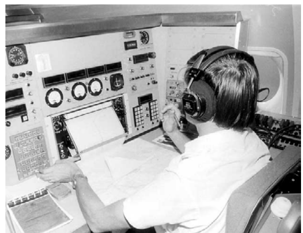
Figure 20. Airservices Australia flight inspection equipment installed in Fokker F28 (courtesy Civil Aviation Historical Society, Inc.)
