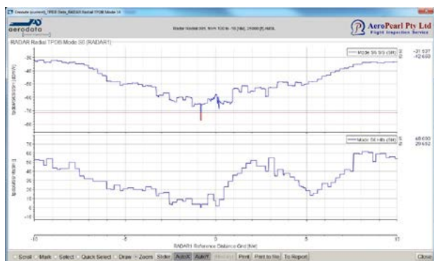
Figure 11 Overhead Cone Check
