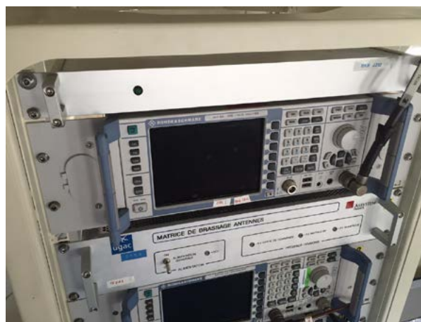
Figure 5. R&S®EDS300 Installation in the FI Aircraft
