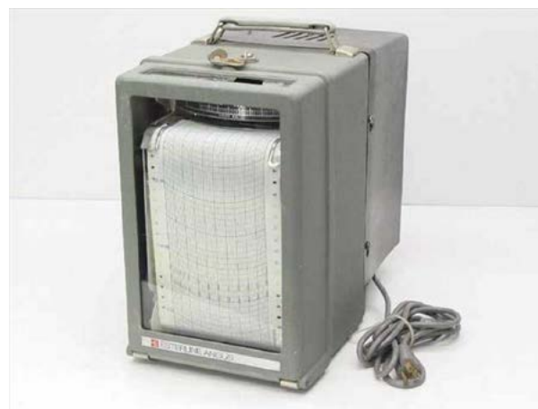
Figure 25. Early pen-type chart recorder (public domain)
