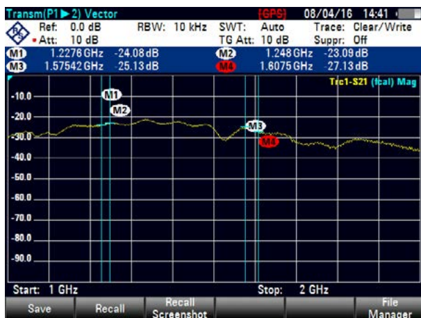
Figure 15 - Typical Passive L-Band Antenna
