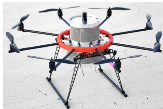
Fig. 2: Photograph of electromagnetically shielded octocopter.
