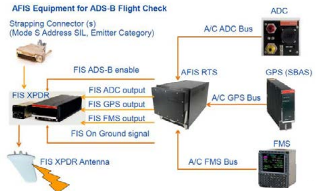
Figure 6: AFIS Configuration ADS-B Out for calibration purposes.
