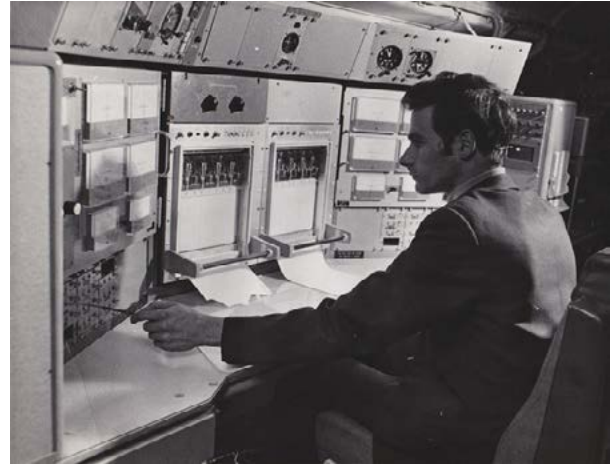
Figure 15. UK CAFU FIS installed on Avro HS-748 aircraft (from Jim Fuller collection)
