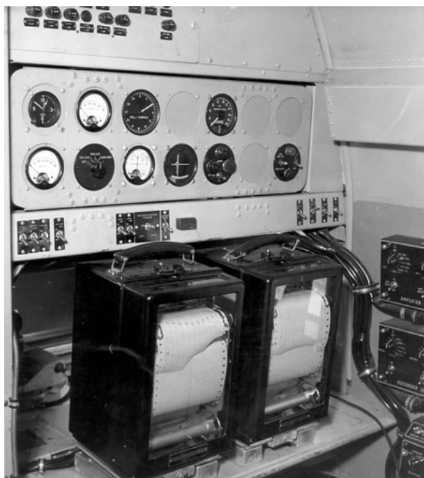
Figure 26. Circa 1954 –Australia DCA flight inspection dual equipment chart recorders (courtesy Civil Aviation Historical Society, Inc.)
