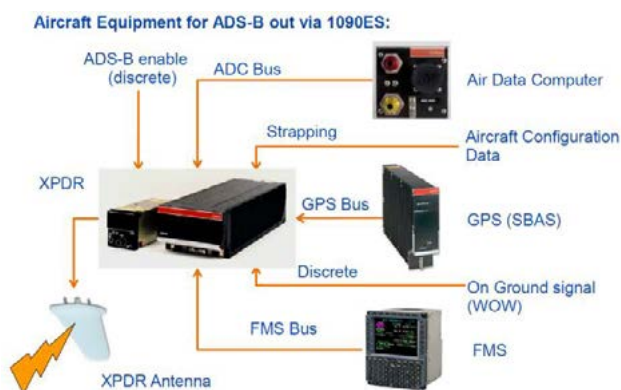
Figure 5: Aircraft Configuration ADS-B Out
