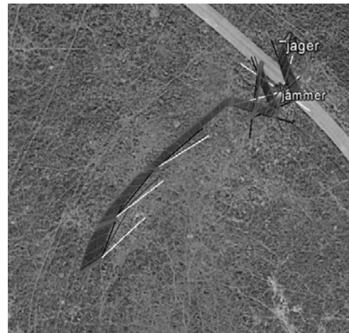
Figure 10. Flight Path of Greedy Path Planning.
