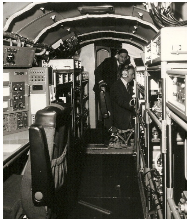
Figure 16. UK CAFU FIS installed on Avro HS-748 aircraft (from Jim Fuller collection)
