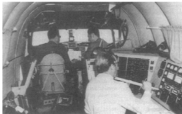
Figure 10. FAA flight inspection equipment installed in DC-3 aircraft (from FAA history office)
