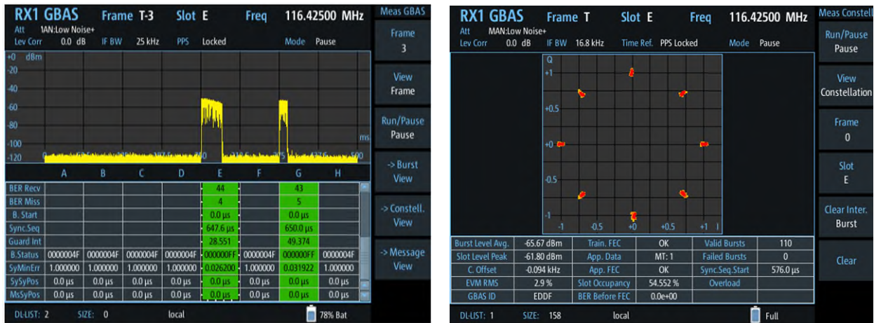
Figure 2. Two bursts of the GAST C VDB displayed by the EVSG1000 (frame view and constellation diagram).
