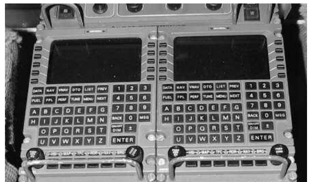
Figure 5. Lear 60 Dual FMSs in Pedestal
