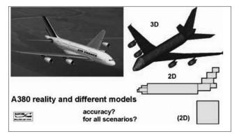
Fig.1: Real object of A380 and different modeling approaches.
