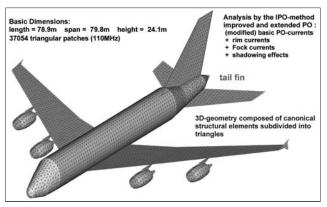
Fig. 2: A380 numerical 3D-model, scattering object.
