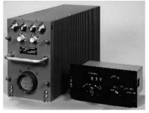
Figure 2: FITACAN Receiver and Control Unit
