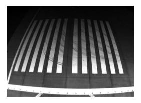
A wider field of view lens will give higher chance of capturing the region of interest even with severe aircraft roll, pitch and heading offsets.
