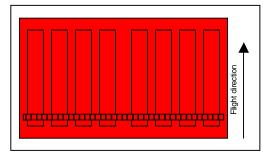
Figure 2 - Line scan camera covers one pixel line at a given time
