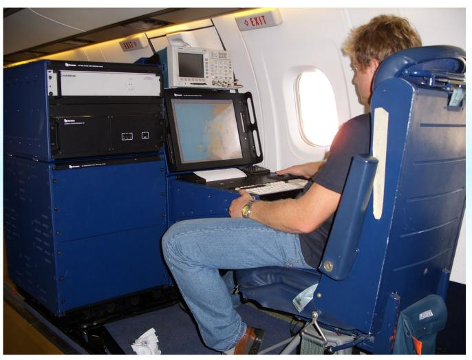
Flight inspection of GNSS-based precision approaches
