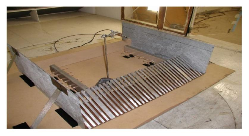
Proto Type Jet Blast Deflector Wind Tunnel Results
