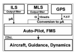
Figure 4. Multi-Mode Receiver feeding Avionics and Aircraft Systems
