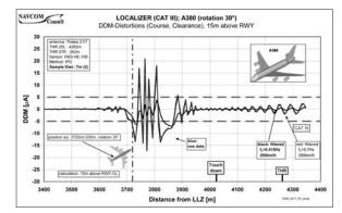
Figure 8. Flight Measurements at 15 Meters, Varying Filter Characteristics, Insufficient Sampling Rate
