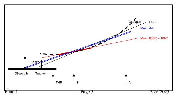
It can be seen from the (exaggerated) diagram above that several interpretations of RDH are possible. Firstly there is the line of glidepath 0ddm, the dashed line on the diagram. There is the arithmetic mean angle as measured by the theodolite system, the double line on the diagram. The Best Fit Straight Line (BFSL) between points A and B, and the TCH as 6000' measured between and 1000', either as an arithmetic mean, or by BFSL.
