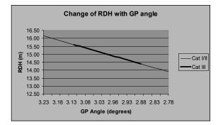
It can be seen that the change in RDH with glidepath angle is significant, even though the glidepath within the remains operating tolerances. Calculated RDH may change by ±1.1m from the nominal with the glidepath remaining within Cat I/II angular operating tolerances, and  $\pm 0.6m$  for Cat III. Can one assume that if the RDH is not less than 15m at the promulgated glidepath angle, the obstacle surface assessment safeguards the operation to the limits of tolerance of the glidepath angle?
