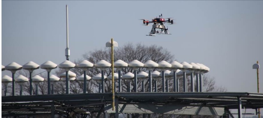
Figure 38: The CNS Drone Conducting a Drone Check
