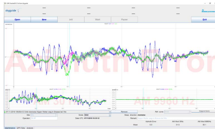
Figure 44: Influence of an External Reflector (different positions)
