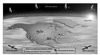
Fig. 1. Wide Area Augmentation System (courtesy of FAA)
