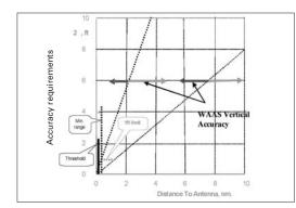
Fig. 3. Comparison of WAAS accuracy and ILS calibration accuracy requirements in vertical
