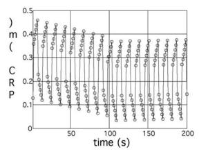
Fig. 7. WAAS fast correction messages
