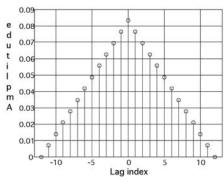
Fig. 9. Impulse response of the low pass filter
