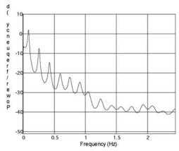
Fig. 6. Spectrum of WAAS airborne noise
