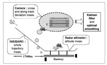
Fig. 2. Position estimation procedure in AFIS
