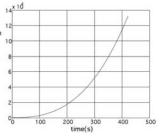
**Fig. 18. Simulated horizontal error for an automotive grade INS** Figure 19 and 20 shows the cross-track errors of the WAAS-Aided FITS using the simulated low-end tactical and the automotive grade INS. In both of the results, the cyclic noise is effectively removed so that it is hard to find any difference between the two cases.
