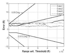
Fig. 15: Cross-track errors of the WAAS-Aided FITS
