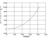
Fig. 17. Simulated horizontal error for a tactical grade INS
