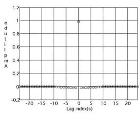
Fig. 11. Impulse response of the high pass filter
