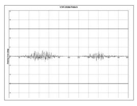
Figure 7. Modeling Results for an Orbital Flight at an Elevation of 1.2 Degrees (5000 ft AGL at 40 nmi).
