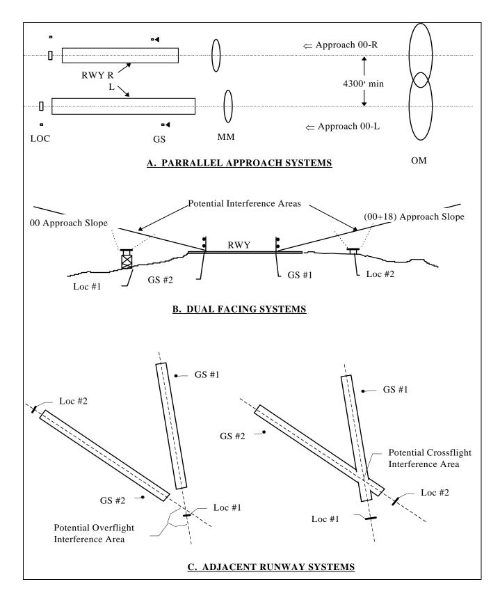
Figure 1. Multiple ILS Configurations
