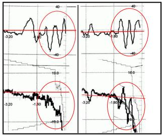
Figure 2. Raw Data (top), with Corrected Data from RTT (bottom left) and DGPS (bottom right).
