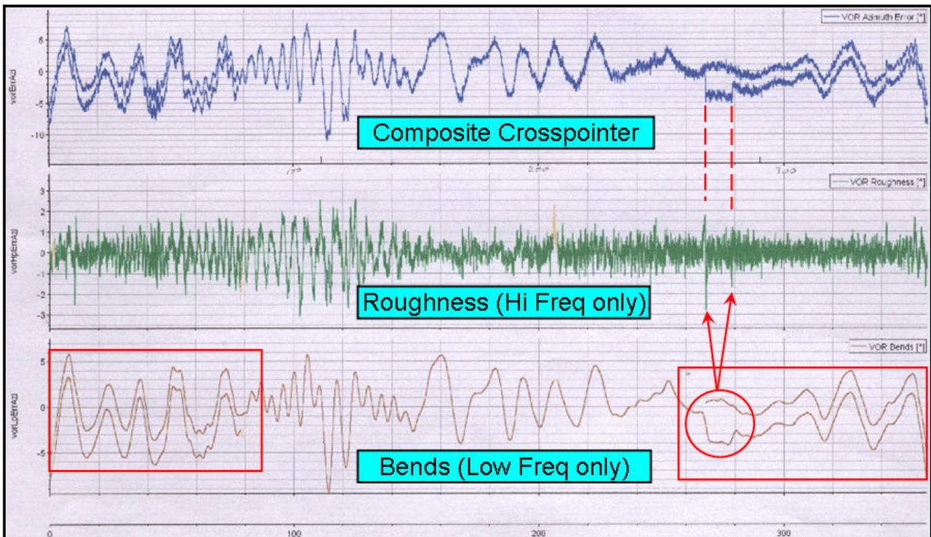
Figure 19. VOR Site Test Orbital Measurements.
