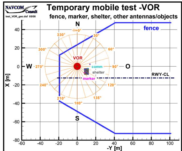
Figure 18. Geometry of the VOR-antenna, airport fence, marker and objects.
