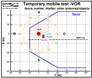
Figure 18. Geometry of the VOR-antenna, airport fence, marker and objects.
