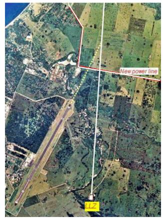
Figure 4. Terrain Avoidance Offset LLZ.
