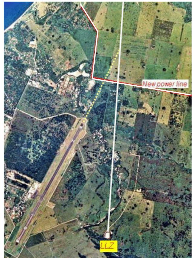
**Figure 4. Terrain Avoidance Offset LLZ.**
