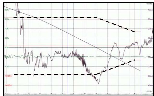
**Figure 5 Out-of-Tolerance Results for Offset LLZ.**
