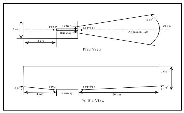
Figure 3. LAAS Approach Coverage Requirements.
