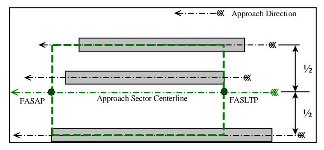
Figure 1. Determining Approach Sector Centerline, FASAP, and FASLTP.
