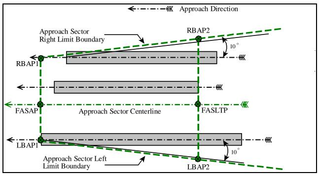
Figure 2. Determining Right/Left Boundary and Boundary Alignment Points.
