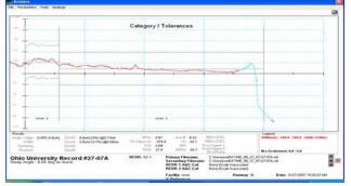
Figure 10. Glide-Slope Path Quality (Category I Tolerances) (Path Angle 6.65 Degrees).[8/27/07]
