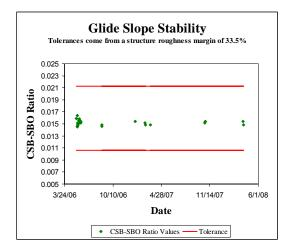
Figure 2011. Confirmation That Path Angle Remained Within Tolerance During Tests -TX Parameters.
