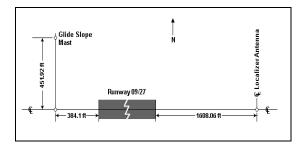
Figure 1. Test Facility Equipment Locations with Reference to Runway 09L at TMB.
