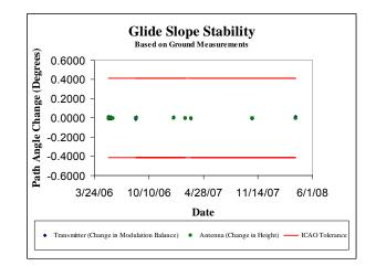
Figure 19. Confirmation That Path Angle Remained Within Tolerance During Tests -TX Modulation and Antenna Height.
