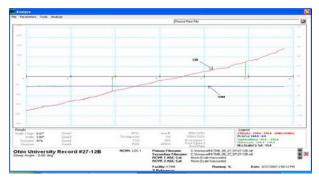
Figure 7. Measured Glide-Slope Guidance Performance (8.65 Degrees). [8/27/07]
