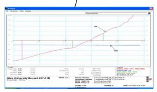
Figure 5. Measured Glide-Slope Guidance Performance (5.5 Degrees).[8/27/07]
