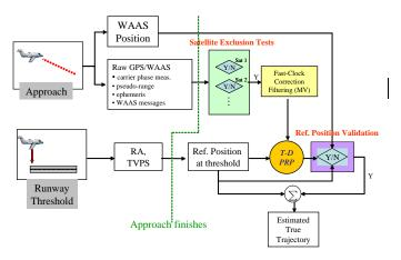
Figure 1: System architecture of the WAAS-based FIS
