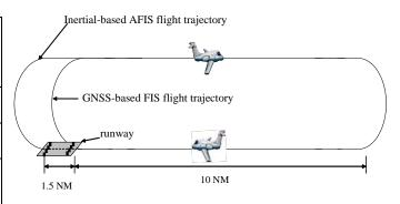
Figure 7: Comparison of flight trajectory using the GNSS-based FIS and the Inertial-based FIS
