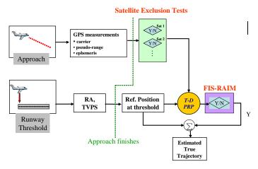
Figure 2: System architecture of the stand-alone GPS-based FIS
