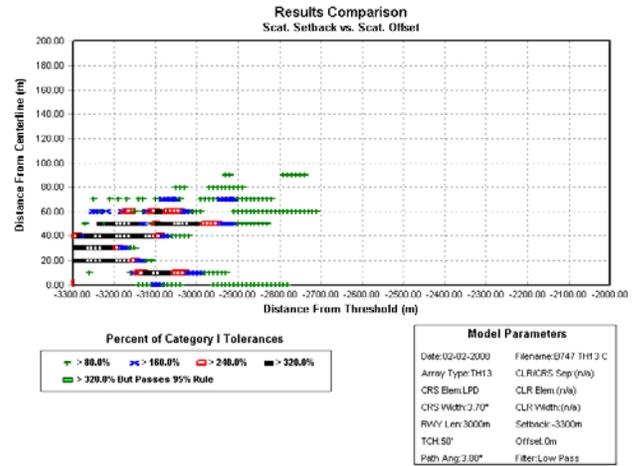
Figure 9. Localizer Critical Area Simulation of B747 Aircraft
