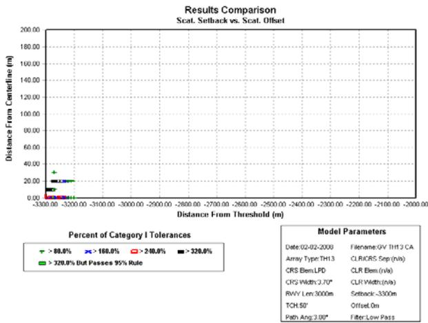
Figure 11. Localizer Critical Area Simulation of GulfStream V Aircraft
