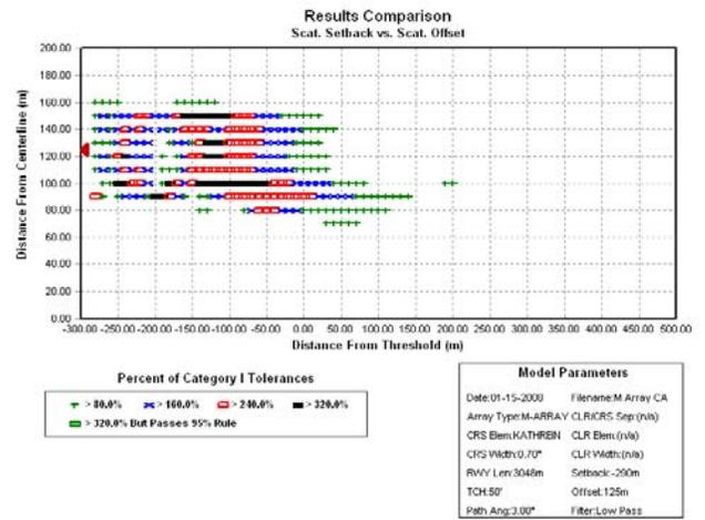
Figure 13. Glide Path Critical Area Simulation of B747 Aircraft
