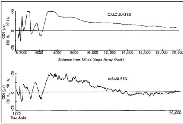
**Figure 2. Glide Path Approach with B747 Positioned 448 Feet from Threshold and 376 Feet from Centerline**
