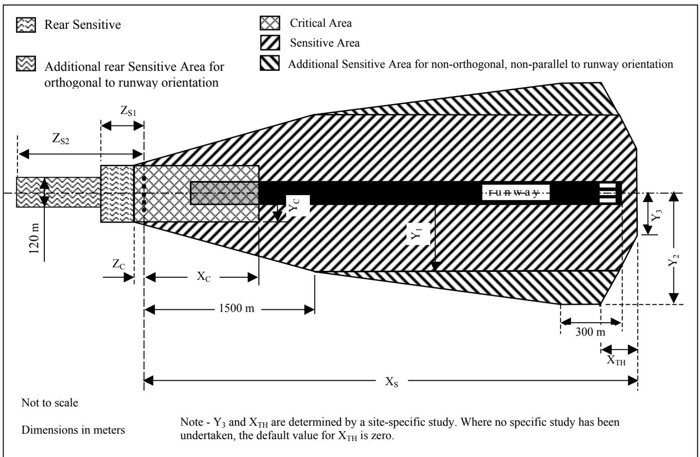
**Figure 16. Diagram of Localizer Critical and Sensitive Areas**
