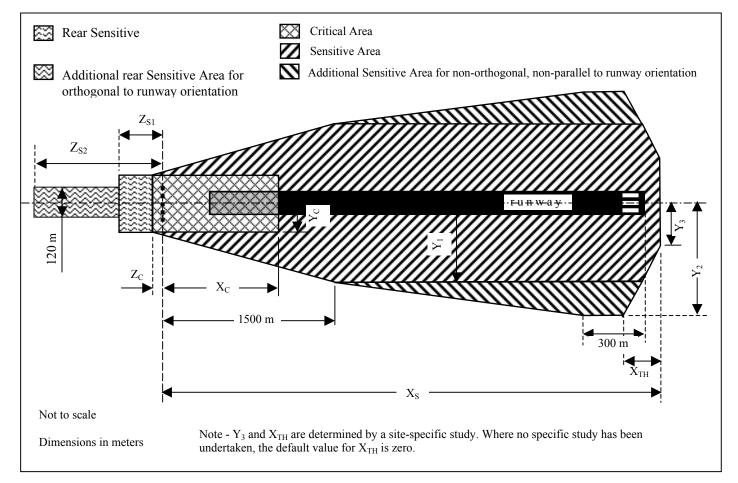
Figure 16. Diagram of Localizer Critical and Sensitive Areas
