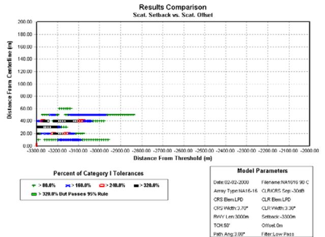
**Figure 5. Critical Area Simulation of B747 with Large Aperture Localizer Array**
