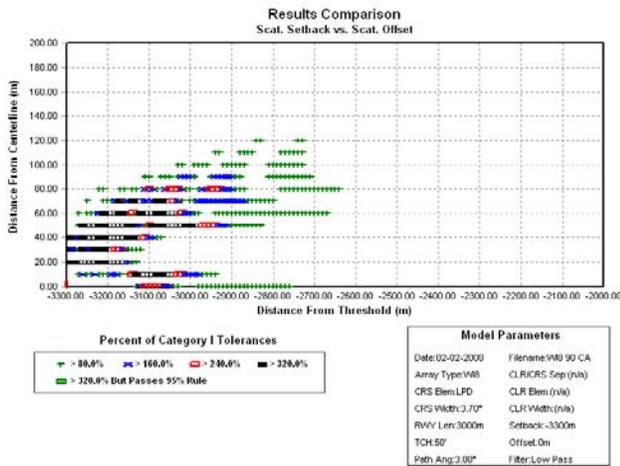
**Figure 3. Critical Area Simulation of B747 with Small Aperture Localizer Array**
