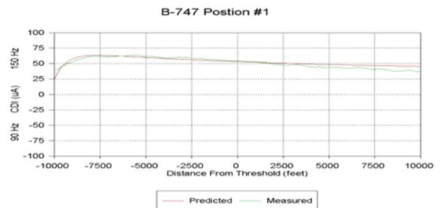
**Figure 1. Localizer Approach with B747 Positioned 1000 Feet from Array and Center of Aircraft 250 Feet Off Centerline with Tail Toward Centerline**
