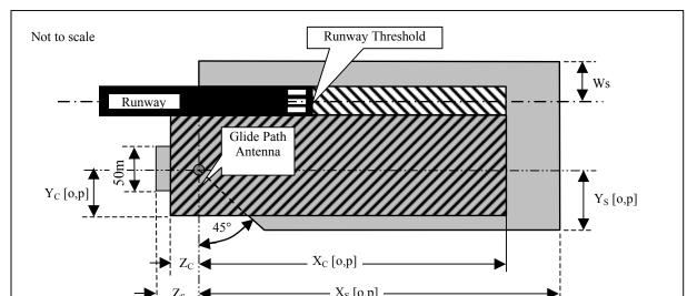
Figure 17. Diagram of Glide Path Critical and Sensitive Areas
