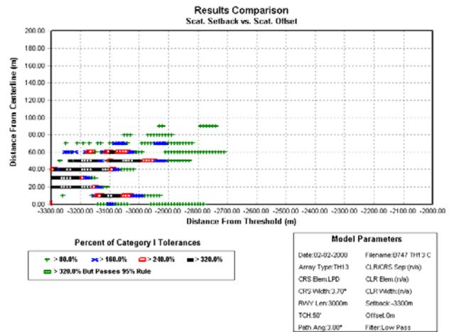
**Figure 4. Critical Area Simulation of B747 with Medium Aperture Localizer Array**
