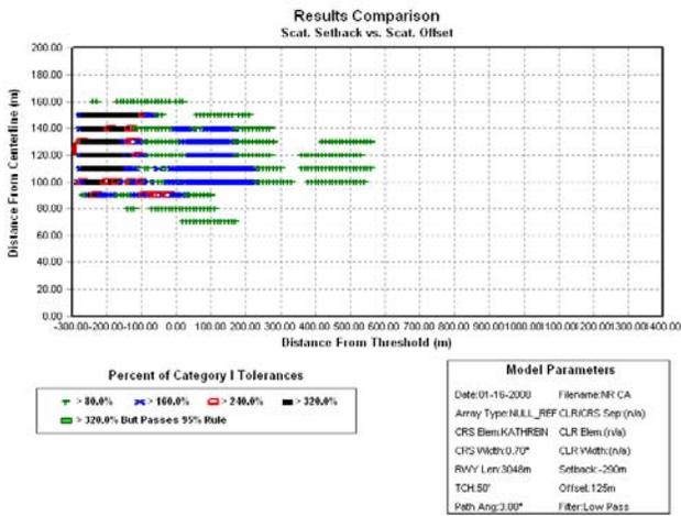
Figure 6. Critical Area Simulation of B747 with Null Reference Glide Path
