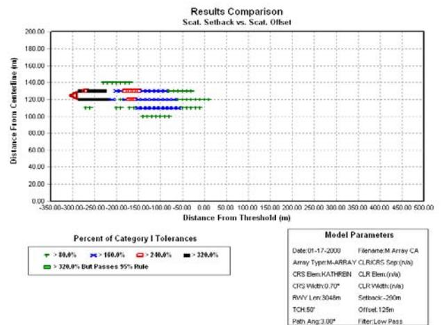
Figure 15. Glide Path Critical Area Simulation of GulfStream V Aircraft
