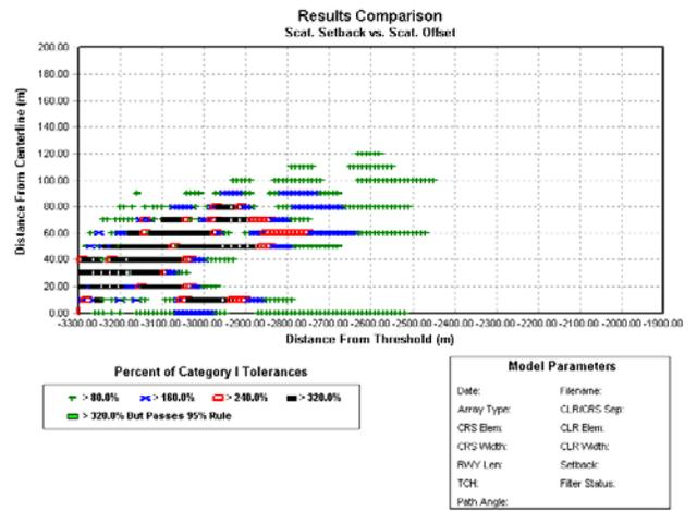
Figure 8. Localizer Critical Area Simulation of A380 Aircraft
