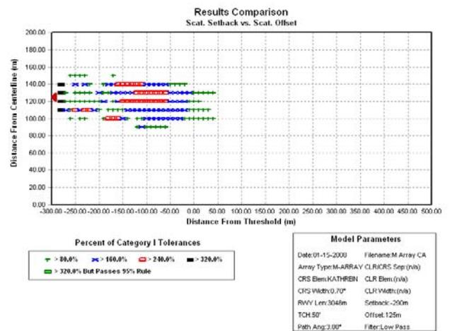
Figure 14. Glide Path Critical Area Simulation of B757 Aircraft
