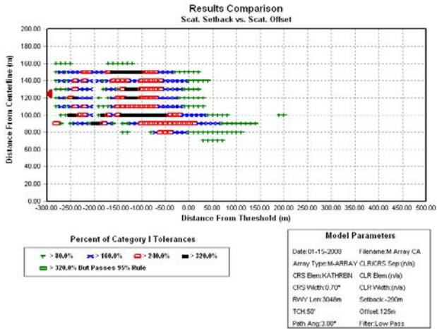
Figure 7. Critical Area Simulation of B747 with M-Array Glide Path
