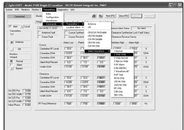
**Figure 8. Transmitter Commands Drop Down Menu**
