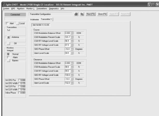
**Figure 2. Localizer Transmitter Configuration Tab**
