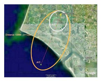
Figure 7: X-Channel Spacing Critical Multipath Ellipses
