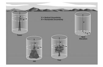
Figure 1 Application of Horizontal and Vertical Accuracy.
