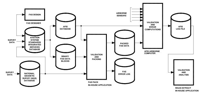
Figure 9. Data Flow – WAAS LPV Flight Inspection
