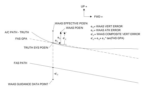
Figure 7. Compensating for ATK Error – Tangent Method
