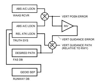
Figure 5. WAAS/LPV Vertical Error and Path
