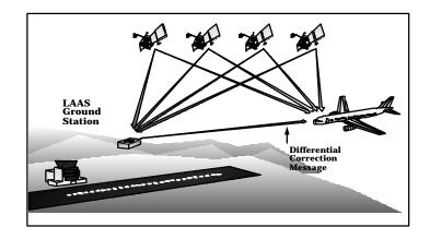
Figure 2-4 Local Area Augmentation System (LAAS)
