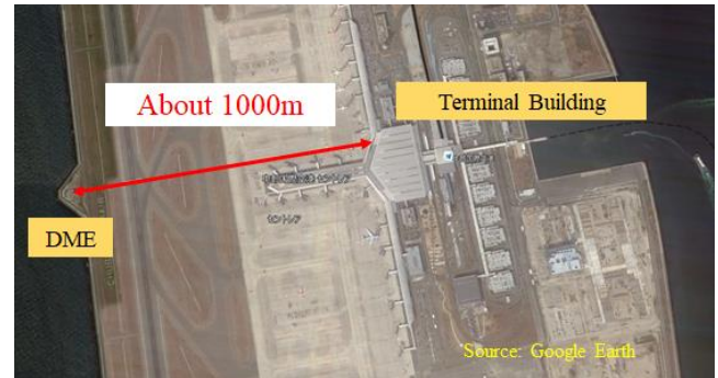
Figure 11. Distance between DME ground station and terminal building
