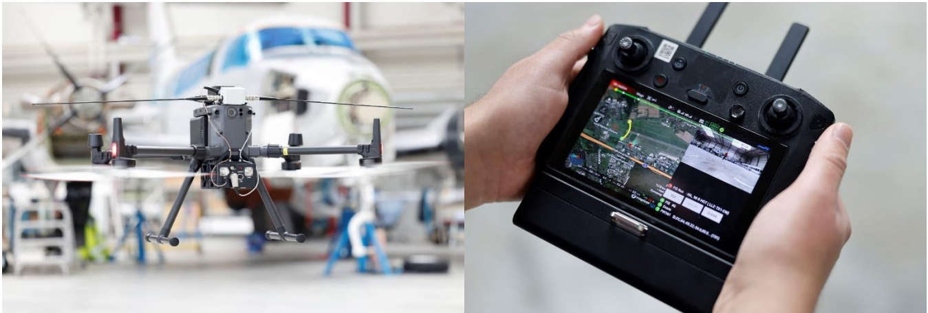
Figure 4: Left: in-door flight of the AeroFIS® Flybot with ILS flight inspection payload Right: AeroFIS® Flybot Remote Control software running on the UAS remote control
